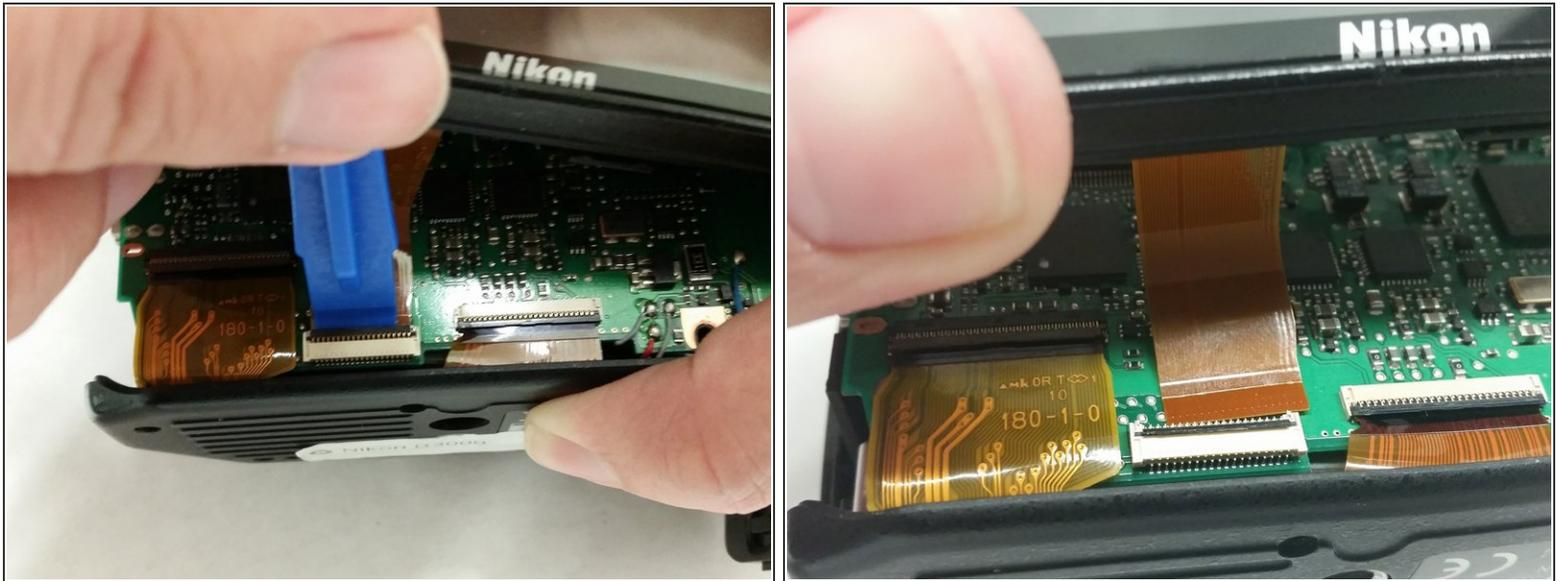
**i** Use the following process for removing all ribbon connectors.
