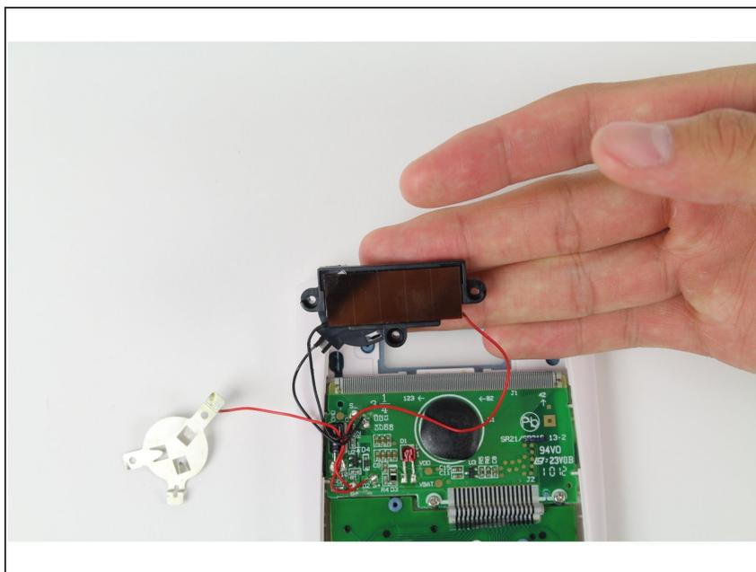
**⚠** Be careful not to pull the solar panel too far out, as the wires connecting it to the calculator are fragile and could be ripped off.
