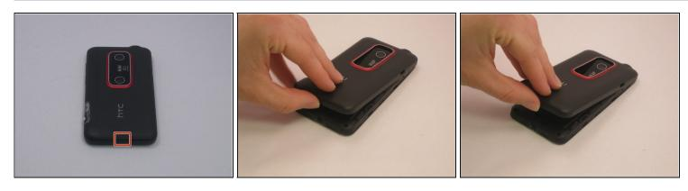
• Remove the outer casing of the phone with your hands by prying and lifting at the latch.
