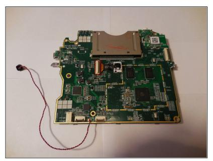
Disconnect the ribbon cable attached to the camera itself by using <u>tweezers</u>.
