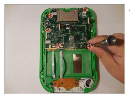
Unscrew the five screws holding the motherboard into the housing.
