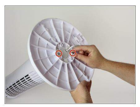
Remove the two 3/4" wing screws on the bottom of the fan by rotating them counter-clockwise.
