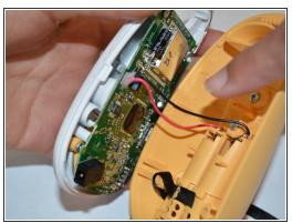
Use a plastic opening tool to gently pry along the middle of the 2 sections of the plastic housing in order to release plastic latches on the inside of the housing.
