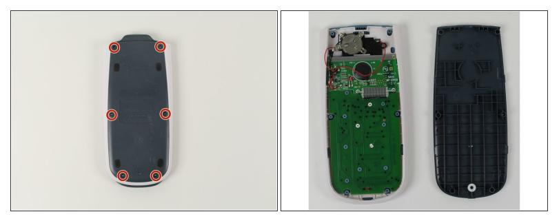
If the screw is not turning, do not force it. This can strip the screw. See the <u>How to Remove a</u> <u>Stripped Screw</u> guide if the screw is already stripped.
