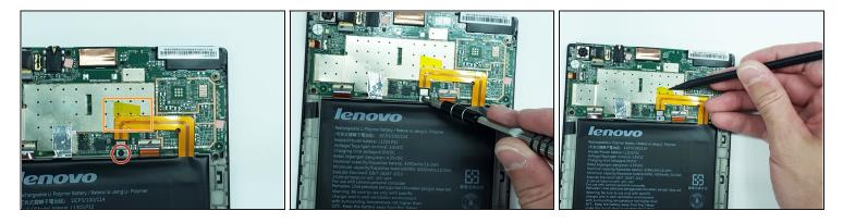
• After removing the cover, remove the M1.6 x 2 mm screw from the battery cable with the JIS J000 screwdriver.
