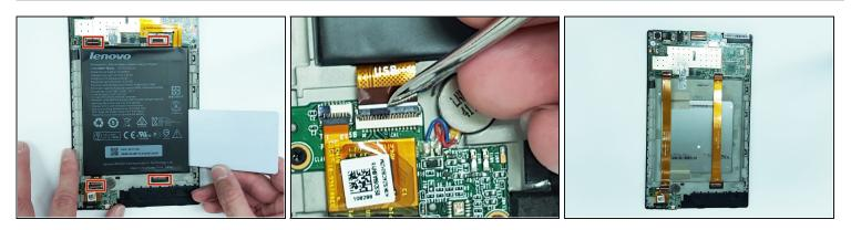
A Before removing the battery, be sure to disconnect the ribbon cables underneath it. The cables might stick to the battery during removal and cause damage.
