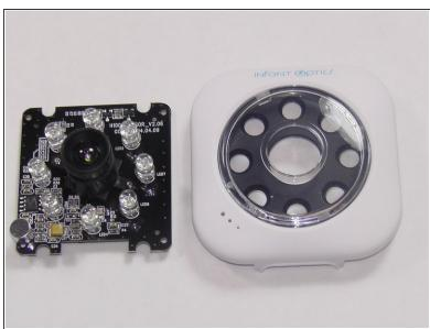
Remove the front face plate of the camera unit by carefully pulling it off.
