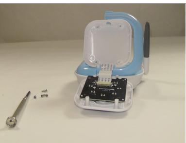
Using a Phillips #2 screwdriver, remove the four, 6.0 mm Phillips screws from the back of the camera unit.
