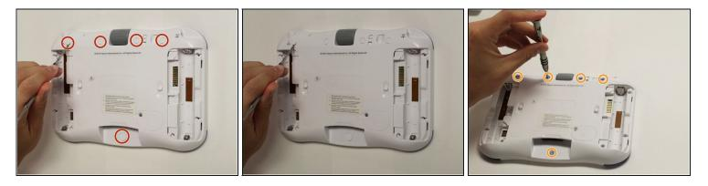
• Using a nylon spudger, remove the five caps that hide the screws.
