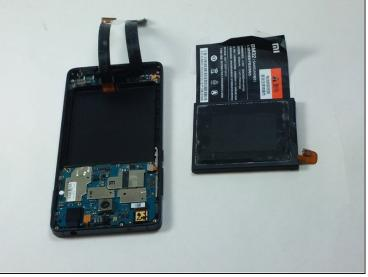
Use the plastic opening tool to gently pry the battery out of its casing for removal.
