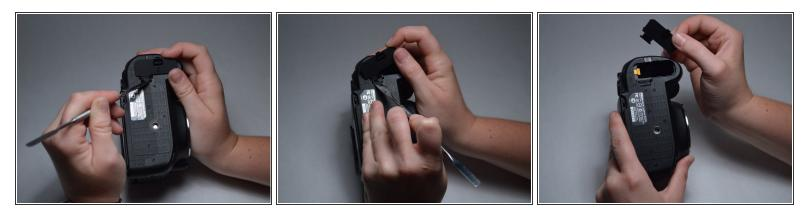
• Using a spudger or other prying tool, gently pop the battery door off of its hinge.
