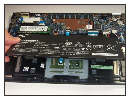
Carefully remove the battery from the device.
