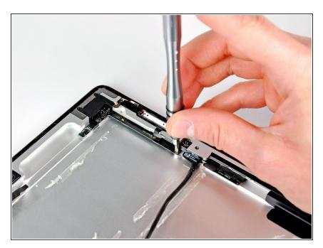
Removing a screw that secures the volume control board to the case.
