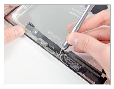
Removing the two screws securing the dock connector to the case.
