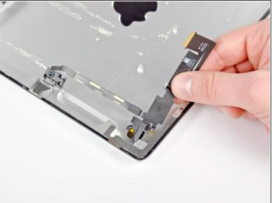
After removing a screw securing the front-facing camera assembly to the case and peeling off a little more adhesive, the assembly can be removed.
