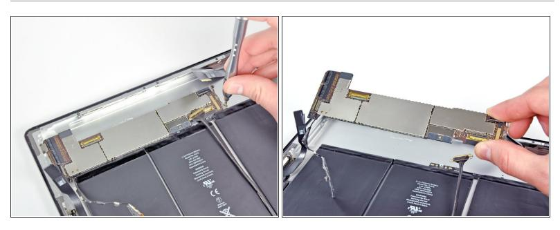
The logic board comes out without a fuss after removing the Phillips screws securing it to the case.
