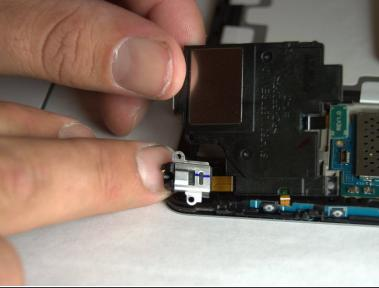
Pull the speaker out and lay it to the side until the rest of the connections are disconnected.
