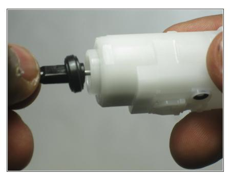
Remove the rubber stopper from the top of the motor shaft by gently pulling it off.
