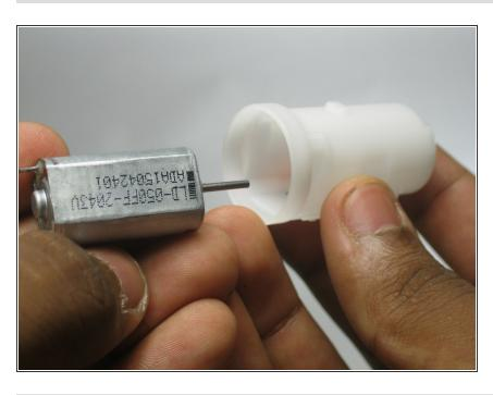
Remove the motor from the case by sliding the cover off of it.
