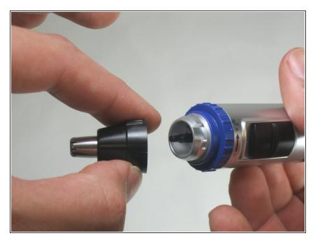
Remove the black trimmer cap from the top of the device by gently pulling it.
