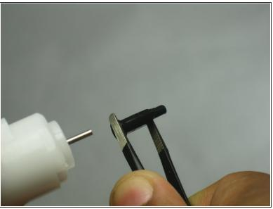
Use a pair of tweezers to remove the plastic cover of the motor shaft by pulling it away from the motor.
