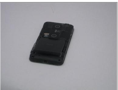
(i) When insert the new battery, be sure to align the golden contacts on the top part of the battery compartment with the replacement battery.
