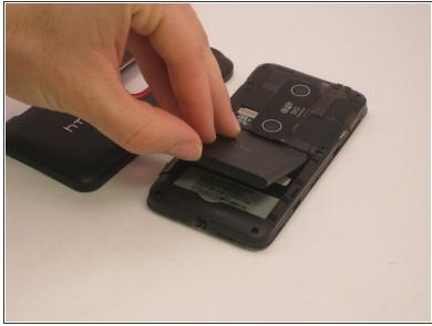
Remove the battery by pulling up on the lower indenture in the battery compartment.
