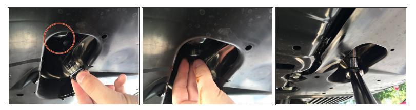
🕢 When reinstalling the oil drain plug, replace the crush washer (part# 803916010) .
