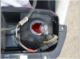
Remove the brake light. Twist the light bulb socket clockwise and remove the light bulb socket from the rear light assembly.
