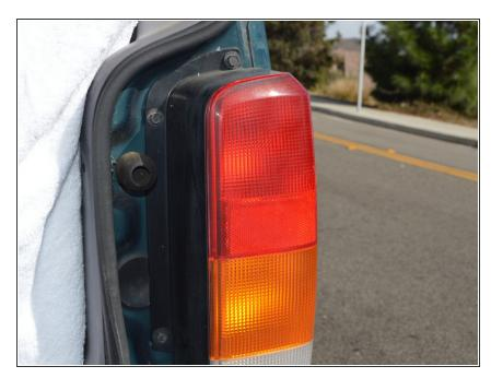
Open the trunk door. In order to remove the rear light assembly, it must be accessed with the trunk open.
