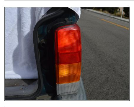
Check the brake light. Have another person step on the brake to ensure proper lighting occurs.
