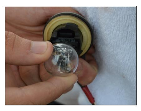
Replace with the new bulb. Gently put in the new bulb in the same manner as you removed the old bulb.
