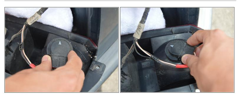
• Lock the bulb back in place. Carefully put the bulb back into the light assembly and twist counter clockwise until it locks in place.
