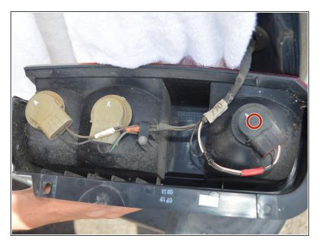
Locate the brake light. Turn the light assembly over and you will see three light bulb sockets. The brake light is the top bulb and the bulb behind the red plastic lens.
