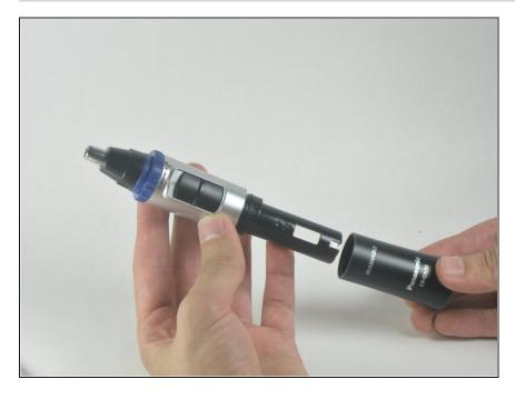
• Remove the back battery cap from the device by twisting it to the unlock position and pulling.
