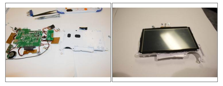
$\triangle$  Avoid forceful movements when separating the screen from the motherboard.
