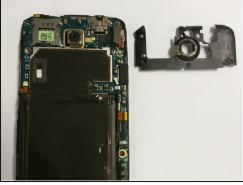
• Remove the five 2.4mm screws located around the camera using a Philips head screwdriver to remove the plastic cover.
