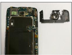
Using a Philips head screw driver, remove the five 2.4mm screws that are pictured. Then remove the plastic cover.
