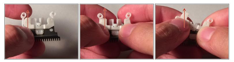
• Remove the plastic casing from the underside of the blade.
