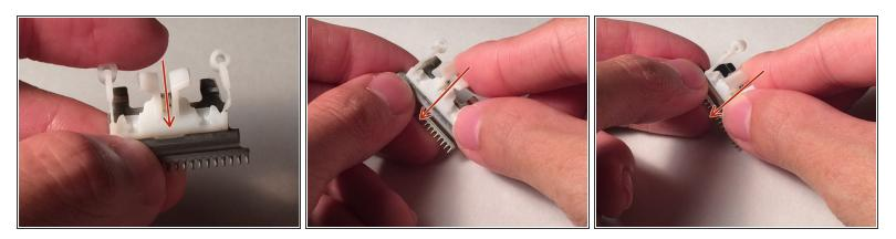
• Remove the last plastic casing from the front side of the blade.
