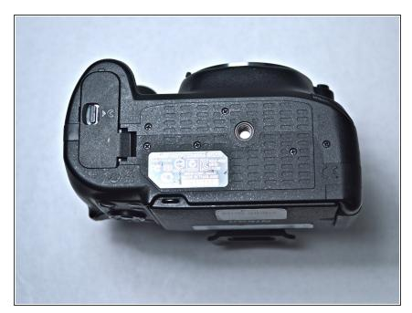
Open the compartment door by sliding the release switch toward the tripod mount and pulling the door outwards.
