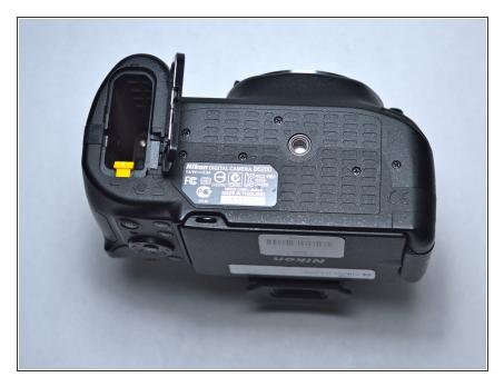
Press the yellow tab downwards to release the battery, and then hold the camera upright to allow the battery to slip out.
