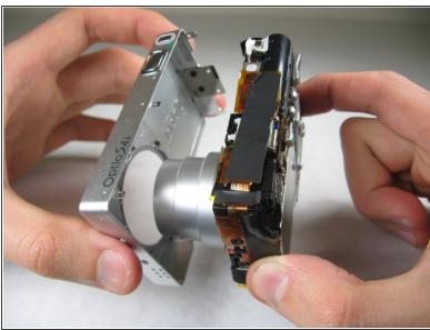
• To remove the front cover, gently hold the inside structure of the camera and slowly pull the front cover off.
