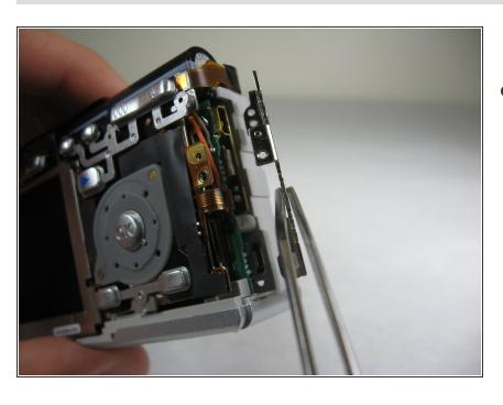
Pull the cover plate off for the two power cord jacks.
