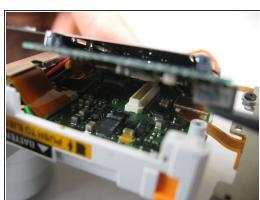
Carefully lift up SD cardholder to reveal logicboard.
