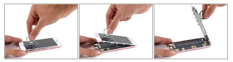
• Use the suction cup to open the display, breaking the last of the adhesive.
