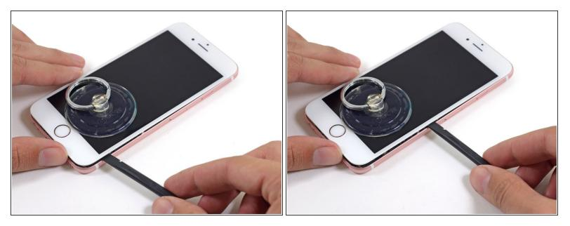
• Use the edge of a spudger to slice through the adhesive on either side of the phone.
