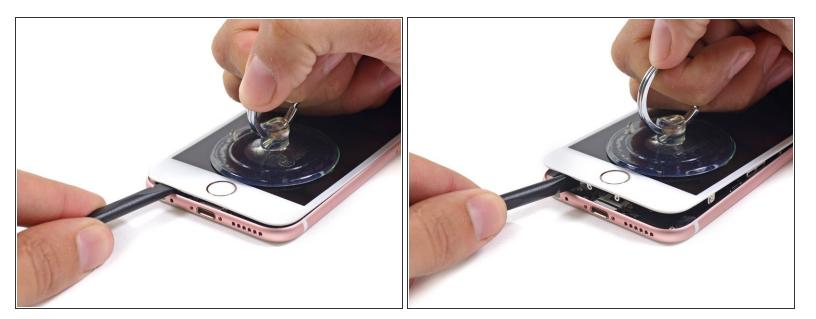
• Twist the spudger to open the gap more and break it free from the adhesive.
