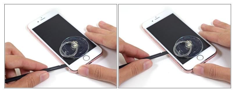
• Use the edge of a spudger to slice through the adhesive on either side of the phone.
