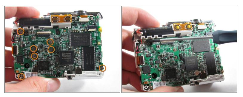
Remove the seven 2.7 mm using a #00 screwdriver.
