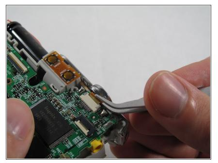
Remove the ribbon cord located near the top right corner of the motherboard. Do this by carefully pulling the cord out of the socket using a pair of tweezers.
