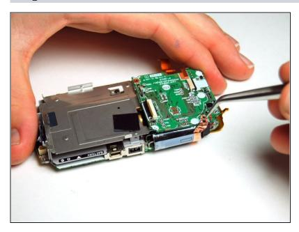
With the tweezers, carefully peel back the copper ribbon that was underneath the black screw.
