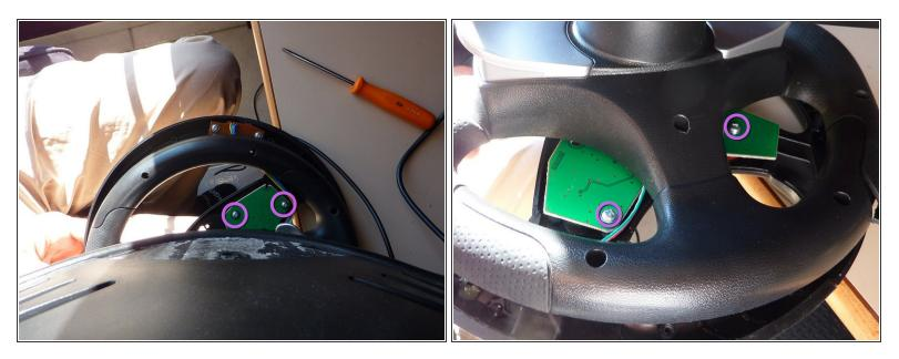
• Put the steering wheel as shown on the photo and unscrew as indicated.
