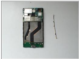
Disconnect the Antenna cable from the Logic board and from the Charging Dock board and remove it.
