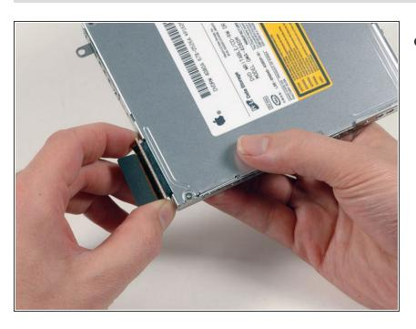
Disconnect the orange ribbon cable from the optical drive.
