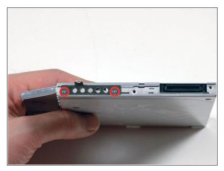
Rotate the drive and remove the two Phillips screws securing the mounting bracket to the rear of the optical drive.
