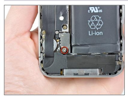
Remove the single 1.5 mm Phillips screw securing the battery connector to the logic board (if present).
