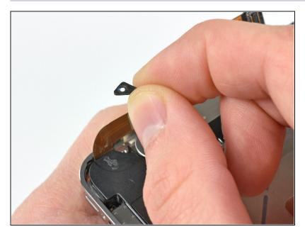
• Remove the small black spacer that was under the Phillips screw near the vibrator.
