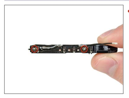
• Remove the two 1.6 mm Phillips screws securing the cellular antenna to the speaker enclosure.
