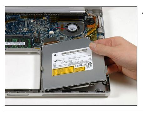
Lift the optical drive up and out of the computer.
