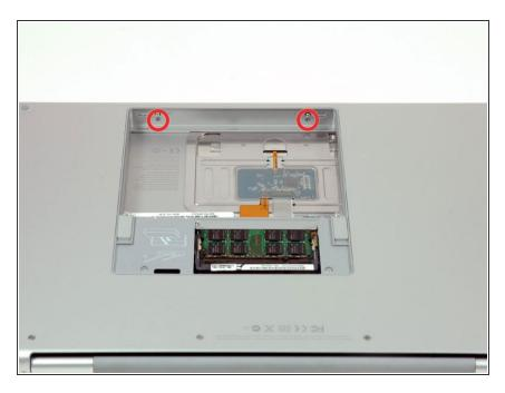
Remove the two Phillips screws in the battery compartment near the latch.
