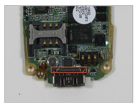
Solder connections are accessable to replace the Chargers Jack.
