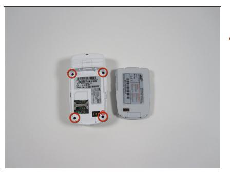
Remove the 4 (4.7mm) philips head screws.
