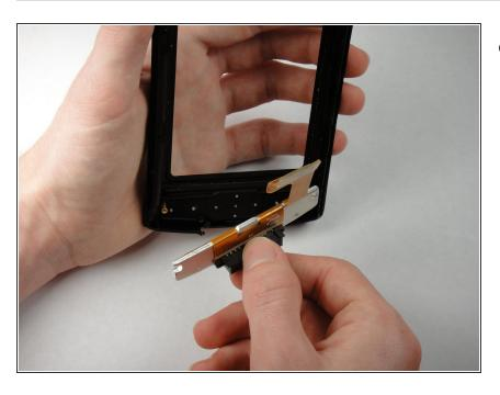
Lift the button and connector assembly from the front panel.
