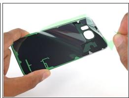
Peel back the inner film layer.
