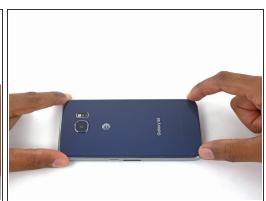
• Lower the rest of the rear panel and press it firmly into the midframe.
