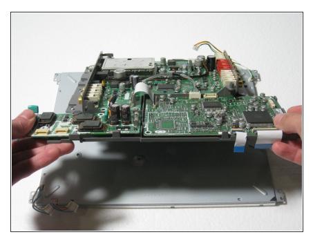
Lift and remove the circuit board from the LCD frame.
