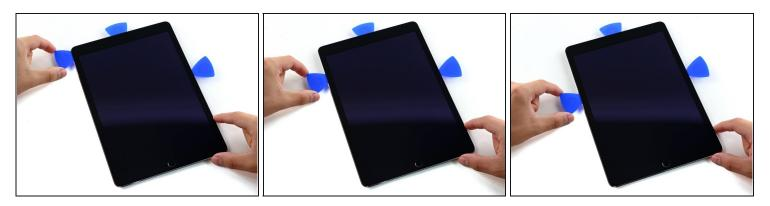
• Slide the left-hand opening pick about halfway down the edge of the display.
