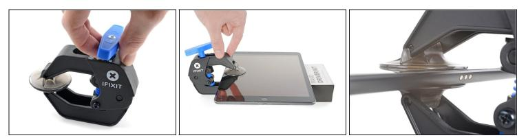
(i) The next two steps demonstrate the <u>Anti-Clamp</u>, a tool we designed to make the opening procedure easier. **If you aren't using the Anti-Clamp, skip down two steps for an alternate method.**
