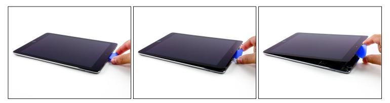
• Twist the remaining pick by the front-facing camera to separate the top edge of the display assembly from the rear case.
