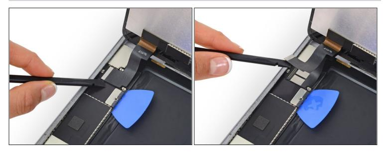
• Disconnect the display data connector from its socket on the logic board.
