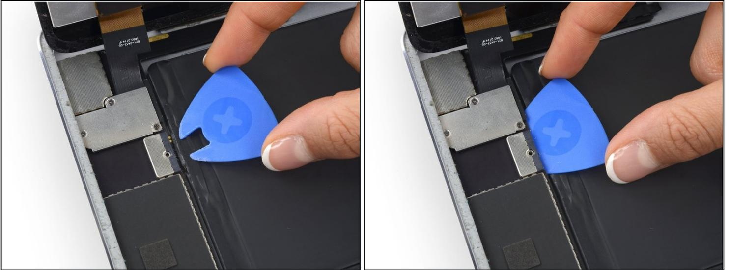
ⓘ To reduce the risk of a short, you can use a battery isolation pick to disconnect the battery.
