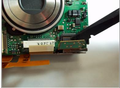
The rest of the ribbon cables are not secured with ZIF connectors. Remove the ribbon cable on the bottom right corner of the motherboard by using the flat end of the spudger to pry the cable from the board.
