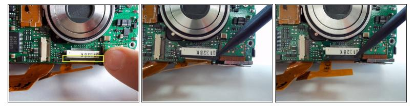
Release the ZIF connector securing the ribbon directly below the lens. To do this, insert the
