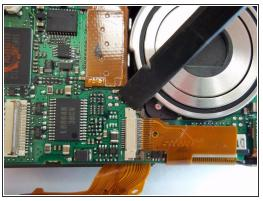
• Release the ZIF connector securing the next ribbon cable. To do this, insert the flat end of a spudger between the dark brown piece and the white piece of the connector. Since the dark brown piece is under the ribbon cable, move this piece to the right by wedging one end at a time.
