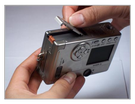
Hold the end of the battery cover that extends beyond the camera and lift it up.
