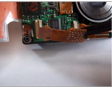
Now, insert the spudger under the ribbon cable and gently pull the cable out of its port.
