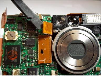
(i) Remove the next ribbon cable by using the flat end of the spudger to pry the cable from the board.
