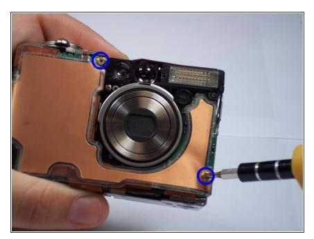
Remove the two 3.9mm screws holding down the copper flap that insulates the motherboard.
