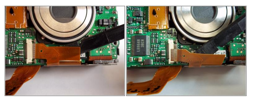
Insert the spudger under the ribbon cable and gently pull the cable out of its port.
