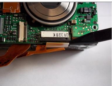
Insert the pointed end of the spudger under the ribbon cable and gently pull the cable out of its port.
