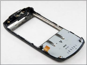
• Using your fingers gently lift the display screen panel out of the casing by either grasping it from the back or popping it out of the front.
