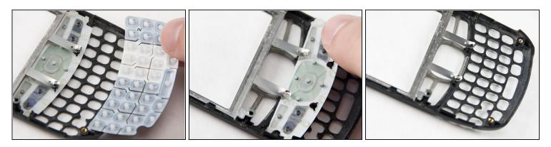
Lift up and remove the rubber keypad and button pads.
