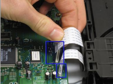
• Remove the two white ribbon cables that connect the motherboard and the disc tray by pulling on the ribbon cable where it attaches to the circuit board.
