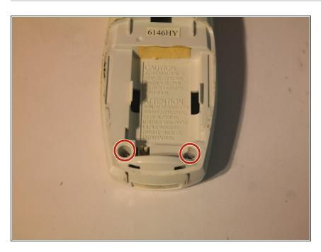
Remove 2 phillips screws inside the battery compartment.
