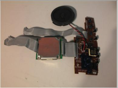
The entire top case assembly can be removed from the printer after using a spudger to free the large buttons from clips in the top case.
