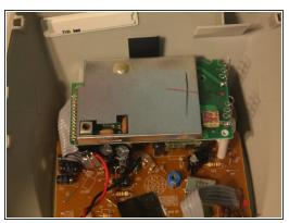
Remove 1 screw to remove the wireless module.
