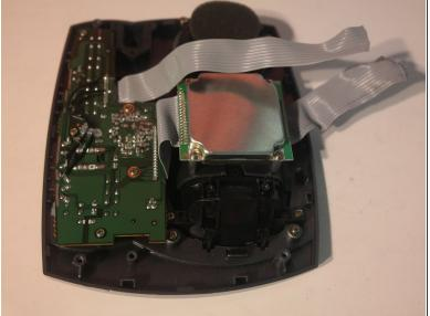
• Remove 2 screws to remove the charging contacts in the upper case.
