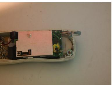
Remove 2 screws on what appears to be the wireless board.
