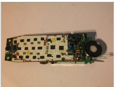
The mainboard assembly can now be removed from the front case.
