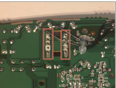
All of the boards in this phone system have terrible solder quality. I was able to cleanly remove the 7-segment display, about 20 capacitors, 3 voltage regulators, 1 transformer, and 2 crystal oscillators without damaging them using needle nose pliers.
