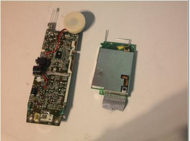
The wireless board is attached by a soldered and hot-glued in ribbon cable, which must be cut off to remove.
