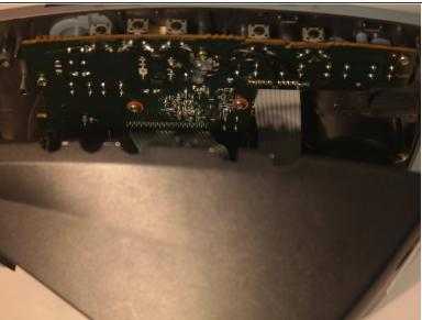
Remove the buttons from the side of the case.
