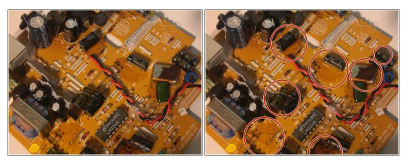
The main board in the base station has patches of an unknown yellowish-brown substance on it that appears to be some kind of weak adhesive, and it seems to be scattered in no obvious pattern.
