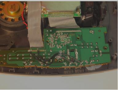
The upper case board can be removed by removing 5 screws.
