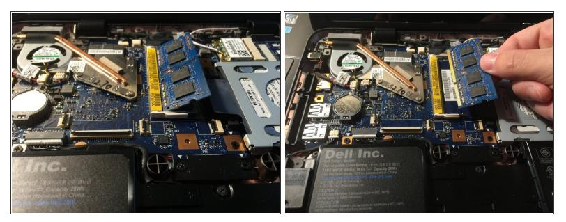
• With the RAM stick flipped up, carefully lift it out of the slot.
