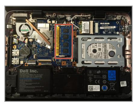
With the cover removed, locate the 2GB RAM stick. It will be in the upper-middle portion of the device. The RAM stick is the flat blue rectangular object that has four black squares running along it vertically (for convenience, the RAM stick has been outlined in red in the photo).
