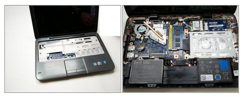
Next, remove the top cover from the device using the plastic opening tools. It snaps in on the sides, so don't worry if you hear it unsnapping; it's not breaking.
