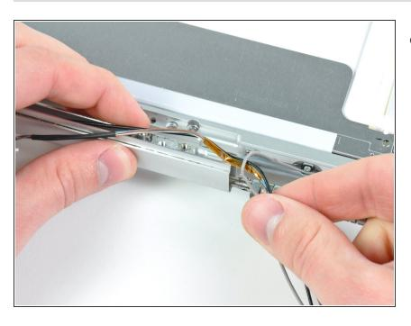
Pull the inverter and antenna cables out of their slot in the clutch hinges.
