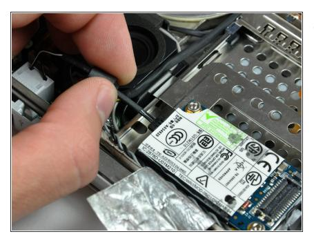
Disconnect the RJ-11 cable from the modem.
