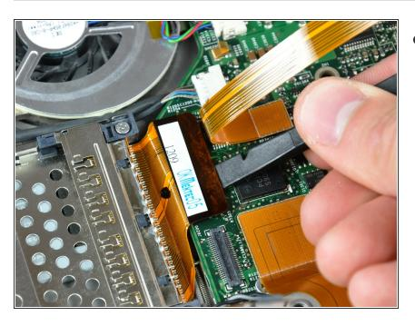
Use the flat end of a spudger to pry the PC card cage connector up off the logic board.
