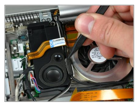
If necessary, use the tip of a spudger to remove the small piece of foam tape from the side of the left speaker.
