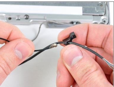
De-route the black and gray antenna cables through the black plastic cable retainer attached to the inverter cable.
