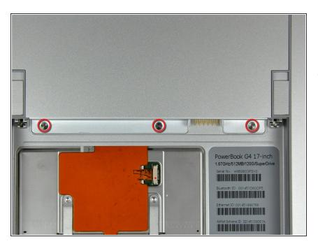
Remove the three 2.3 mm Phillips screws securing the memory cover to the lower case.
