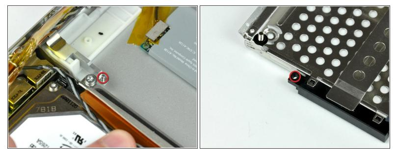
When reinstalling your PC card cage, be sure to insert the post sticking up from the PC card release button into the hole in the black plastic release mechanism on the PC card cage.
