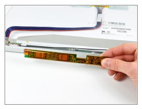
Remove the inverter from the display.
