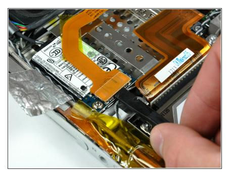
Use the flat end of a spudger to pry the modem cable connector up off the modem.
