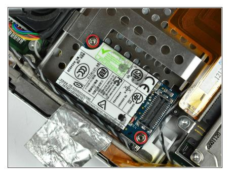
Use a 4 mm nut driver to remove the two nuts securing the modem to the PC card cage.
