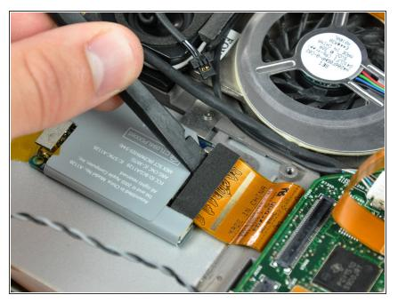
Use the flat end of a spudger to pry the ribbon cable connector up off the AirPort/Bluetooth board.
