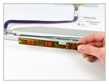
• Remove the inverter from the display.
