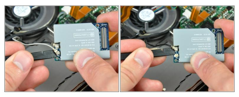
• Use the flat end of a spudger to pry both antenna connectors up off the AirPort/Bluetooth board.
