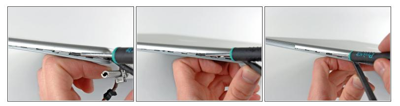
• Insert the flat end of a spudger between the front display bezel and the plastic rim attached to the rear bezel near the lower right corner of the display.
