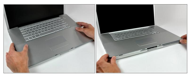
Starting near the display, lift the upper case straight up off the lower case, minding any cables that may get caught.
