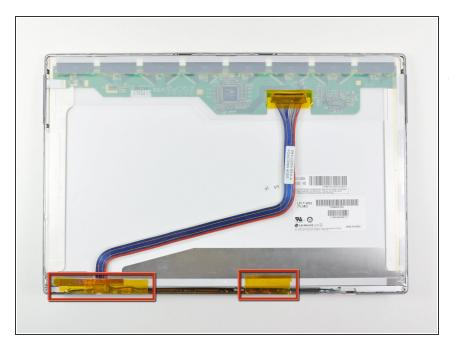
(i) If present, remove the pieces of tape along the bottom edge of the LCD.
