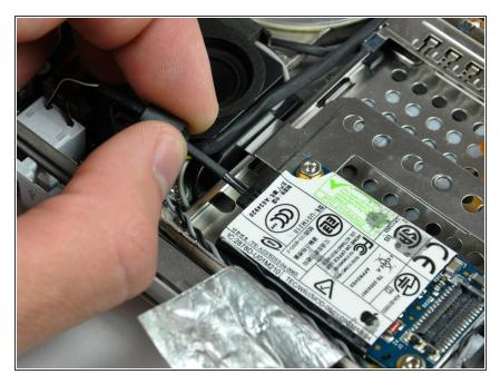
• Disconnect the RJ-11 cable from the modem.
