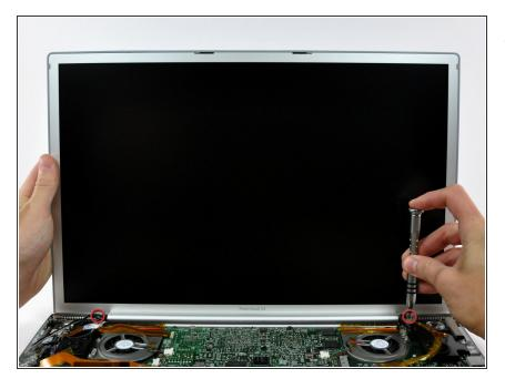
While supporting the display with one hand, remove the one remaining T6 10 mm Torx screw from each display bracket (two screws total).
