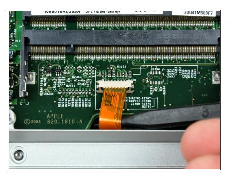
Use the tip of a spudger to slide the trackpad ribbon cable out of its socket.
