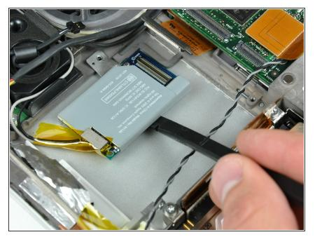
Use the flat end of a spudger to pry the AirPort/Bluetooth board up off the adhesive securing it to the lower case.
