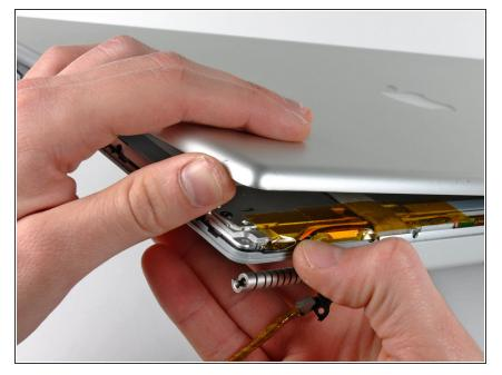
Slightly lift the recently-freed corner of the rear display bezel to separate the clips along the span of the clutch hinges.
