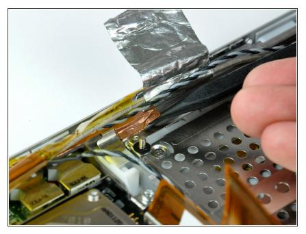
• Use the tip of a spudger to peel back the small strip of copper tape off the edge of the PC card cage near the side of the lower case.
