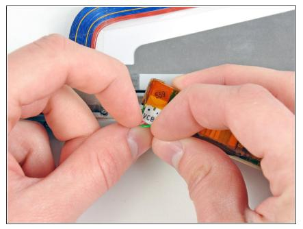
• Disconnect the backlight cable from its socket on the display inverter.
