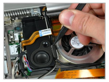
If necessary, use the tip of a spudger to remove the small piece of foam tape from the side of the left speaker.
