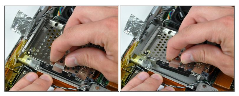
• Lift the PC card cage by its center piece and maneuver it out of the lower case.
