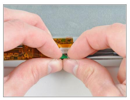
• Disconnect the inverter cable from its socket on the display inverter.
