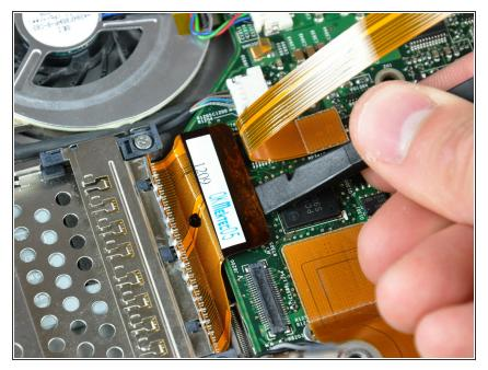
• Use the flat end of a spudger to pry the PC card cage connector up off the logic board.
