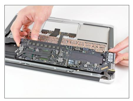
Carefully remove the logic board assembly from the upper case, minding any cables that may get caught.
