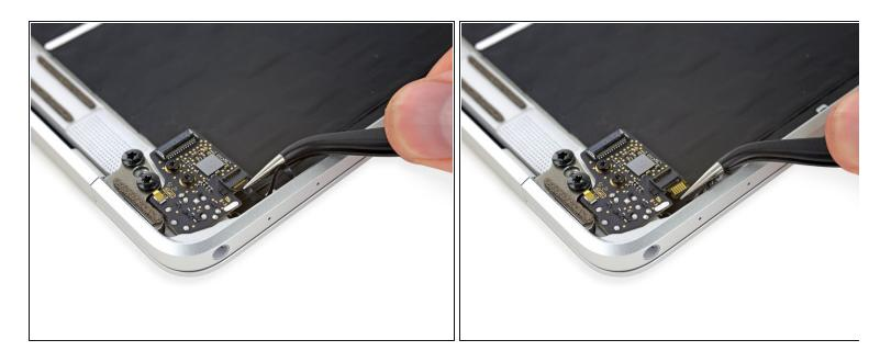
• Use tweezers to pull the microphone assembly ribbon cable free of its connector.
