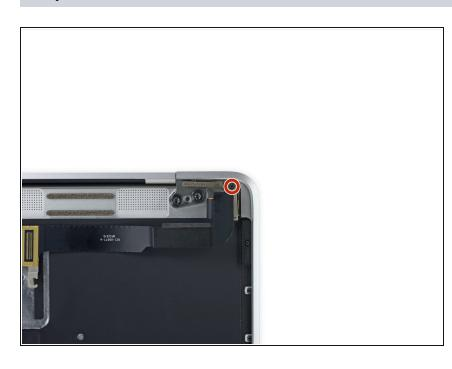
Remove the single 4.3 mm Phillips #00 screw securing the USB-C port ribbon cable.
