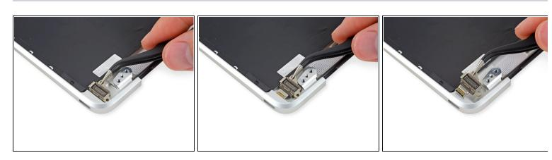
Slide the USB-C port out of its recess in the upper case, and remove the USB-C port.
