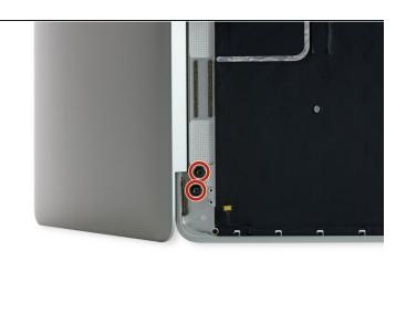
Remove the four 4.8 mm T8 Torx screws securing the display hinges.
