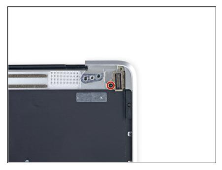
Remove the single 2.9 mm T3 Torx screw securing the USB-C port to the upper case.
