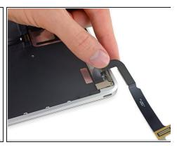
• Unfold the USB-C port ribbon cable until it lays flat, allowing access to the bracket beneath.
