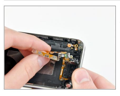
Gently pull the headphone jack electronics away from the side of the rear panel to reveal the plastic mute switch.
